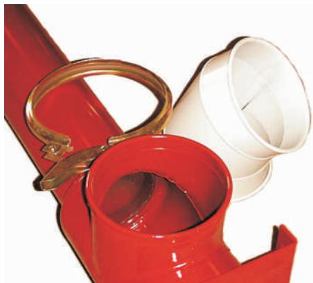
The discharge opening is Ø 160 mm in all models.
